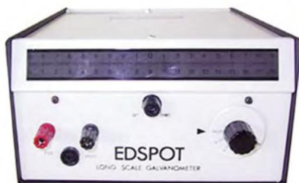
**GALVANOSCOPIO****A MAGNETE MOBILE****4661.00**
